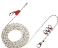
MAS HA4 rope Material: 16 mm twisted rope, polyester Product No.: 130981 13 m with 1 carabiner 130982 16 m with 2 carabiners 130983 20 m with 2 carabiners 130984 23 m with 2 carabiners 130985 25 m with 2 carabiners 130986 30 m with 3 carabiners
